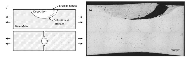
**Figure 7. a)** Side and top view schematic of crack location relative to deposition geometry and **b)** cross-sectional OM image of a lightly etched specimen tested until the initial fracture of the deposited material
