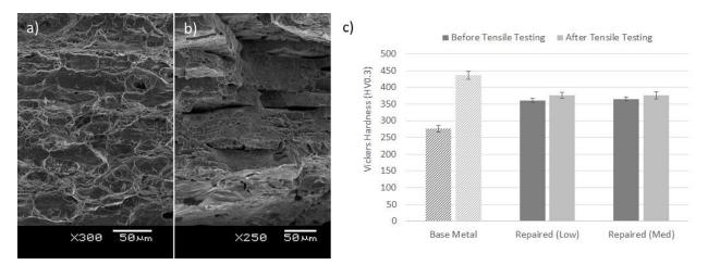
**Figure 5.** SEM image of **a**) base metal fracture surface, **b**) deposition fracture surface with step facets, and **c**) microhardness measurements and standard error of base metal and deposition in repaired specimens within 300 μm of the fracture interface before and after tensile testing
