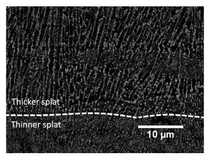
Figure 3. SEM image of subgrain microstructure in ESD processed Inconel 718 after etching
