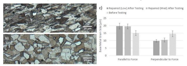
**Figure 6.** Grain structure of Inconel 718 base metal **a**) within 300  $\mu$ m of the fracture interface, **b**) as received prior to testing and **c**) the grain size and standard deviation in the base metal before and after tensile testing within 300  $\mu$ m of the fracture interface
