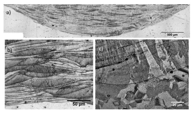
**Figure 2.** Cross sectional OM image after etching of **a**) a repaired cavity, **b**) the deposition splats within a repaired cavity (one splat highlighted with dashed lines) and **c**) epitaxial grain growth (one epitaxial grain highlighted with dashed lines) in deposited material influenced by the substrate base metal grain
