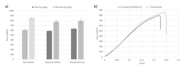
Figure 4. a) Yield and ultimate strengths with standard error and b) representative stress-strain curves
